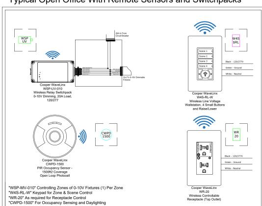
Typical Open Office With Remote Sensors and Switchpacks
